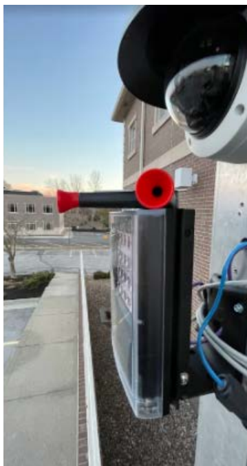
Raytec's DST (Daytime Setup Tool) allows installers to see where the light will illuminate at night
