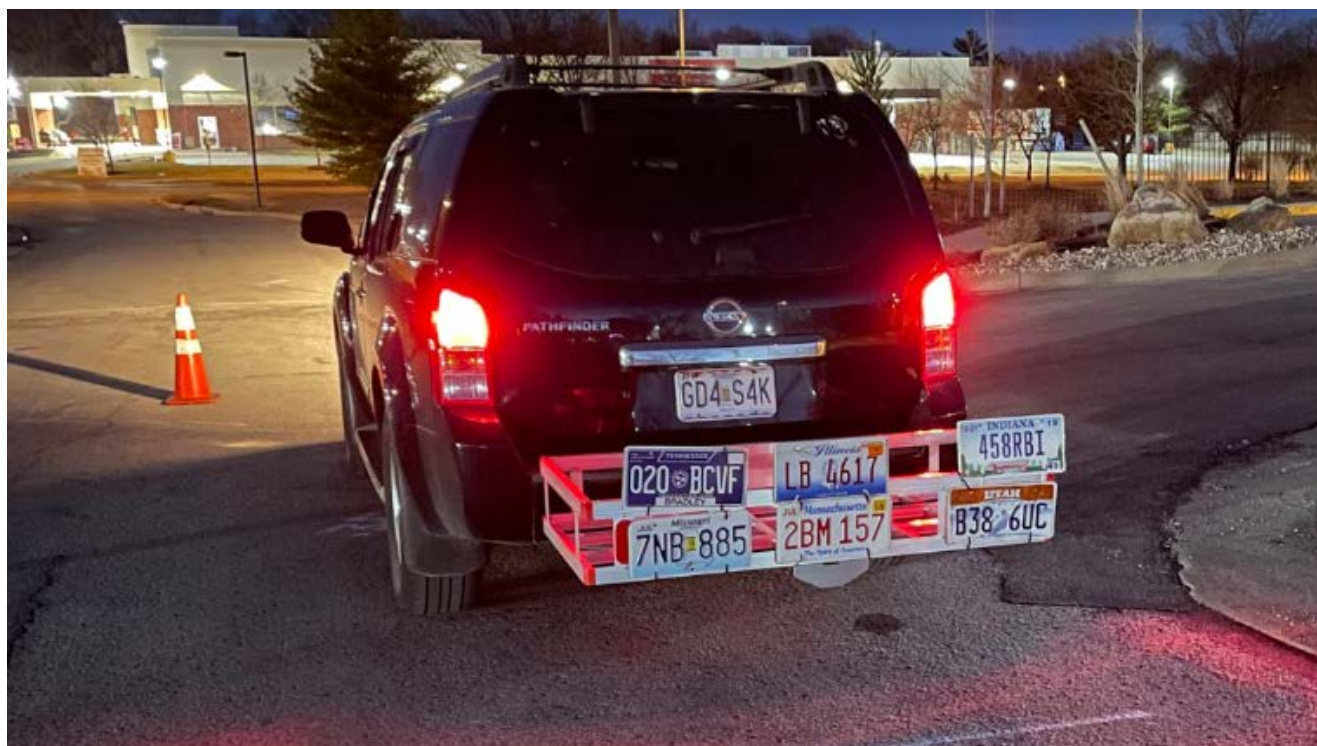
Comparing retro-reflective and non-retro reflective plates. Tennessee and Indiana are in the top left and top right.
