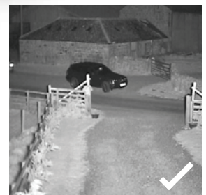
Angle of Illumination Aligned to Camera FOV - Evenly Illuminated. No Over Exposure
