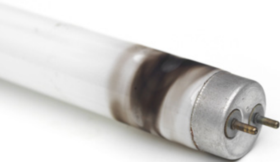
End of life fluorescent tube showing signs of degradation
