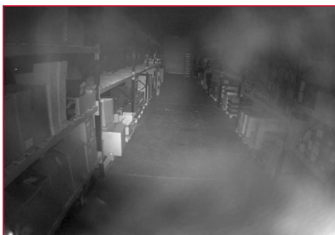
Reflection issues using cameras with in-built IR
