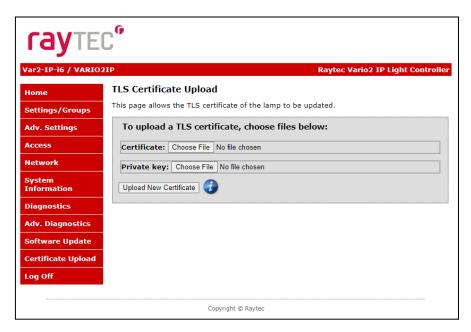
The user must upload a certificate file and private key, these files must be in .der format as this makes the files smaller and allows them to be uploaded and stored in a timely manner.
