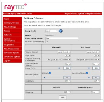
WARNING: For changes to take effect, the SAVE button must be pressed
