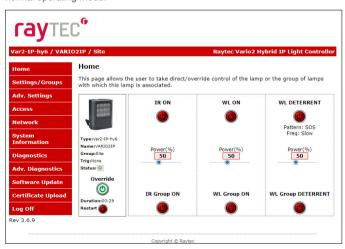
**Important** - If an illuminator is in group override control from another illuminator you will not be able to access the override control on that illuminator.
