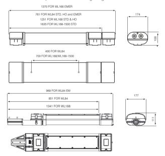
When installing the SPARTAN luminaire vertically where possible, the cable glands should be kept to the bottom of the luminaire.
