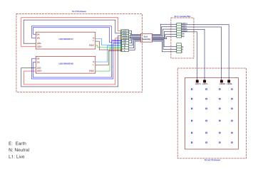
Wire the Mains cable into the terminal block. Provision has been made for this and identified as the E (Earth), L1 (Switched Live), L2 (permanent live) and N (Neutral) terminals. There are two pairs of contacts for each of these to facilitate a mains cable that can be looped in and out of the unit. The L2 terminals on a standard unit are not electrically connected but allows them to be used on the same circuits as emergency bulkheads.
