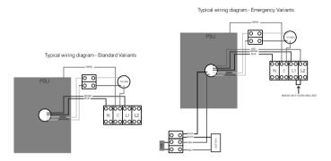
Wire the Mains cable into the terminal block, Provision has been made for this and identified as the E (Earth), L1 (Live switched), L2 (Live permanent) and N (Neutral) terminals. There are two pairs of contacts for each of these to facilitate a mains cable that can be looped in and out of the unit. The L2 terminals on a standard unit are not electrically connected but allows them to be used on the same circuits as emergency bulkheads.
