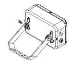
POSITION STIRRUP TO PREFERRED ANGLE AND SECURE USING REMAINING M6 SCREW, SPRING-WASHER AND NUT (ITEM 9)
