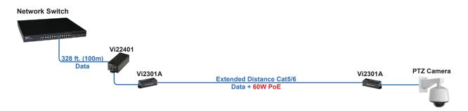
The Vi22401 can send up to 60W PoE power to high power IP cameras at long distances using Vigitron Ethernet and PoE extenders.
