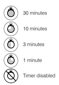
Note: The timer only functions when the Telemetry Input Wires are used with a remote switch; alarm system; PIR detector, etc and a closed circuit input signal is received. The light will come on and stay on. When the input signal stops the light will remain on for the time set by the timer.
