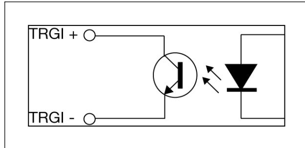
The trigger output can be used to switch a signal of up to 24V, switching up to 20mA when on. When the output is logic 1 (on) a current of up to 20mA can flow. The maximum current must be limited to an absolute maximum of 50mA by the external circuit. The forward voltage is less than 2V.
