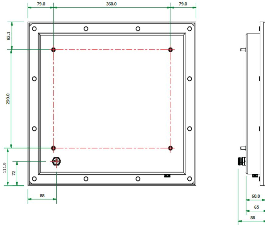
The VTR6 has 4 off M8 mounting studs. These should be fitted to the VTR6 optional mounting bracket, or through 9.0mm diameter holes in the user's infrastructure and fastened with nuts that are tightened to a maximum of 15Nm. If larger diameter holes, or a higher torque is used, then there is a risk of damaging the VTR6.
