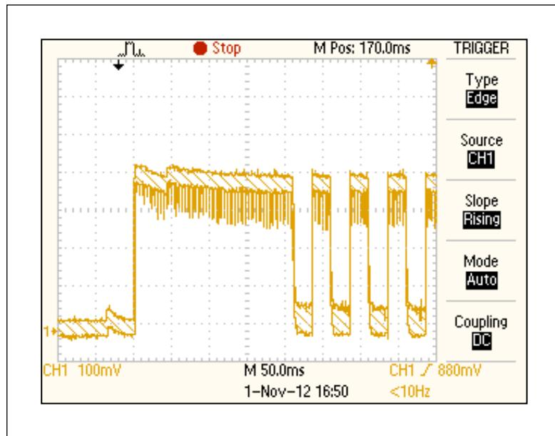
**Note:** The peak of these current pulses is typically 8 Amps, and the mean current consumption is typically 8 Amps once the power-up sequence is complete, and the VTR6 is running at maximum brightness and duty cycle
