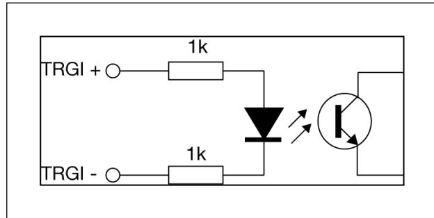
The trigger input circuit operates as follows:
